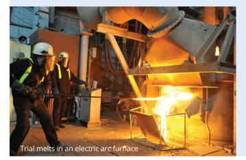
Dr Dunant discovered that the chemical composition of used cement is virtually identical to that of the lime-flux used in the conventional EAF steel recycling process. Traditional Portland clinker, one of the main ingredients in cement, is produced by firing limestone and other minerals in a kiln at extremely high temperatures (1,450 degrees Celsius), a process that accounts for more than 50% of the cement sectors' emissions.
